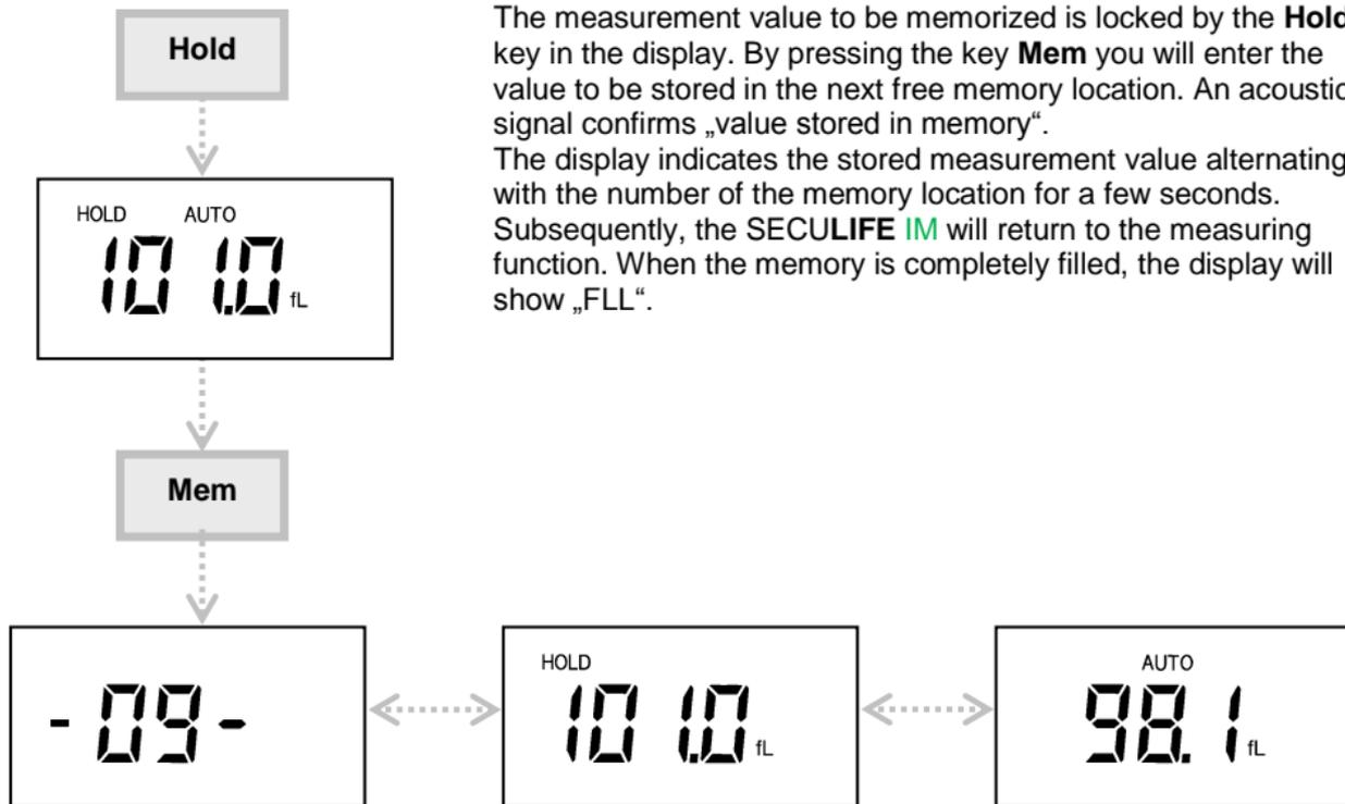
The measurement value to be memorized is locked by the **Hold** key in the display. By pressing the key **Mem** you will enter the value to be stored in the next free memory location. An acoustic signal confirms „value stored in memory“.
