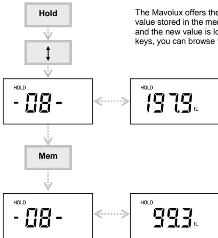
The Mavolux offers the function „Mem Edit“ for correcting a value stored in the memory. Measure again, press the **Hold** key and the new value is locked. Then by pressing one of the range keys, you can browse through the memory.
