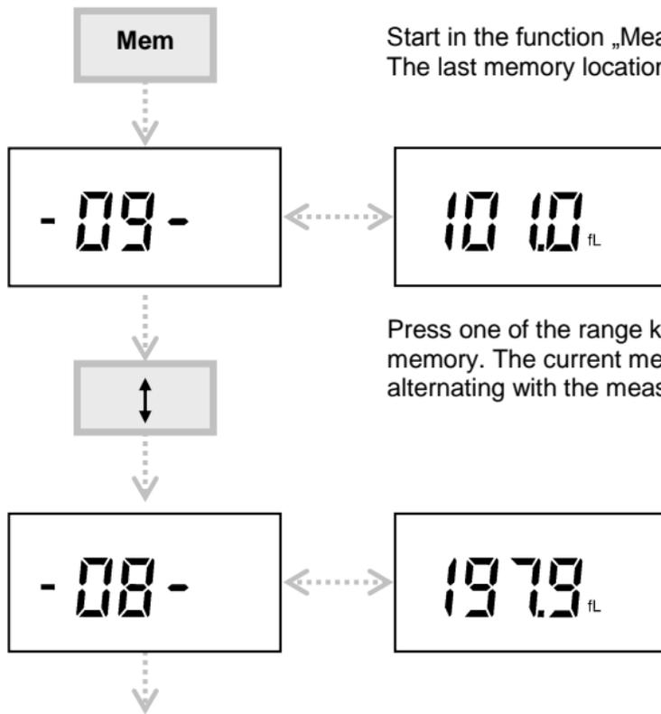
Start in the function „Measuring“ and press the key **Mem**. The last memory location filled will be indicated first.
