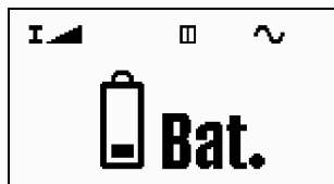
Figure 3.9: Battery Status After Pressing the START Key
