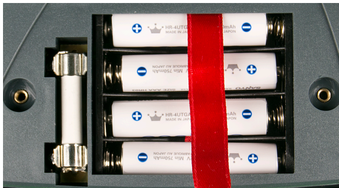
Figure 5: Correct Battery Polarity
