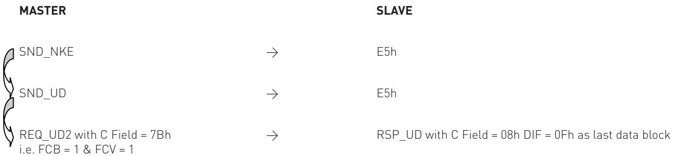
This means that, if the FCB is handled (i.e. FCV = 1), when the RSP\_UD answer has a single-frame of data, the Slave has to send a RSP\_UD answer with the last data block equal to 0F.
