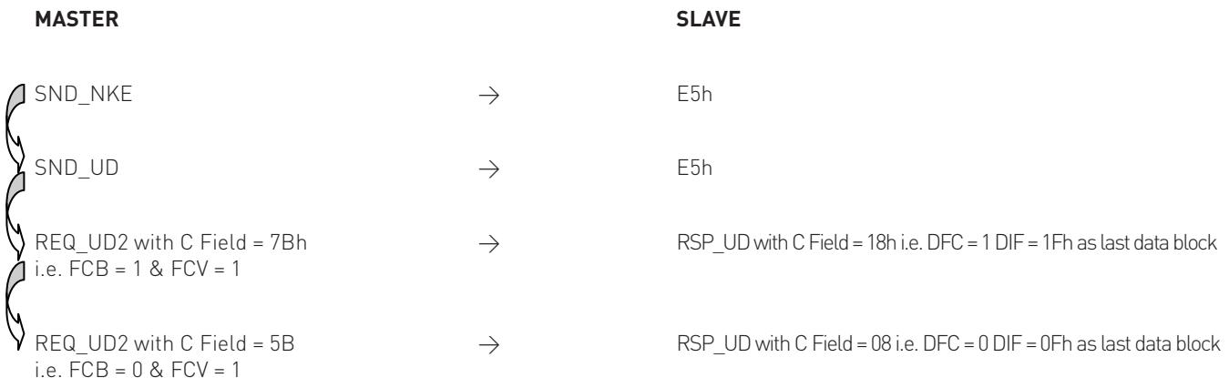
This means that, if the FCB is handled (i.e. FCV = 1), when the RSP\_UD answer has a single-frame of data, the Slave has to send a RSP\_UD answer with the last data block equal to 0F.
