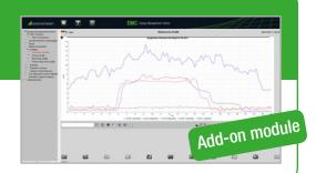
**Export Interface** — all kinds of data can be saved in various types of formats with the help of this module. This allows for the data to be fed into higher-level software solutions where they can be flexibly processed.
