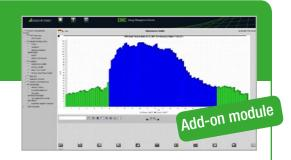
**Industy Billing** — This module makes it possible to read out energy consumption by cost center (e.g. for industrial operations) and by tenant (e.g. for rental properties).
