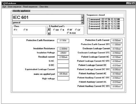
Test results (measured) are also included in the list of test regulations and test specifications. The test results are contained in report templates which can be edited via the "Test result" menu. Branching is established to the "Test result" menu by double clicking a report template.
